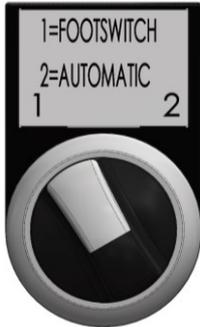
When using 1=FOOTSWITCH the lid will remain closed after the vacuum cycle. If the foot switch (see picture below) is pressed, the lid will automatically open and will close on the other side. After the vacuum cycle, the foot switch can be pressed again, and therefore the movement of the lid is controllable.
