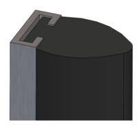
If one of these bumpers is pressed, the automatic movement will stop and the reset button will light up. Be aware that the lid will not stop immediately, but will still move a few centimetres due to momentum. After pressing the reset button the lid can be manually closed after which the automatic movement is continued.
