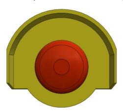
If one of these is pressed, the automatic movement will stop and the reset button will light up. **Be aware that the lid will not stop immediately, but will still move a few centimetres due to momentum**. After pulling the emergency button back out and pressing the reset button the lid can be manually closed after which the automatic movement is continued.
